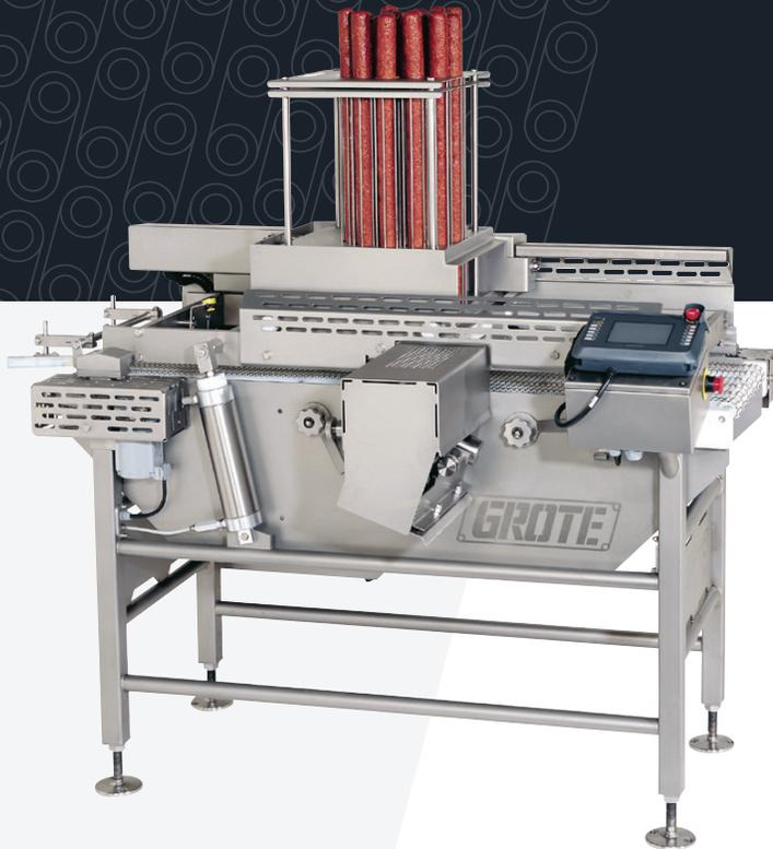
The Peppamatic slices and applies pepperoni directly onto your pizza line, in a variety of patterns and crust sizes. Precise targeting provides consistent accuracy and product quality. Our patented AccuBand® razor sharp, strong band blades cut through product cleanly. The Peppamatic's user-friendly operation and sanitation allow for fast set-up, function selection and thorough cleaning.
